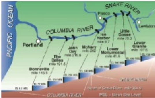
The dams and locks on the Columbia and Snake rivers help maintain a navigation channel that remains at least 14 feet deep for 360 miles between Vancouver, Washington, and Lewiston, Idaho. The system is like a series of elevators that allow barges to navigate the river system, which starts at sea level in Astoria, Oregon, and climbs to 738 feet above sea level in Lewiston.
