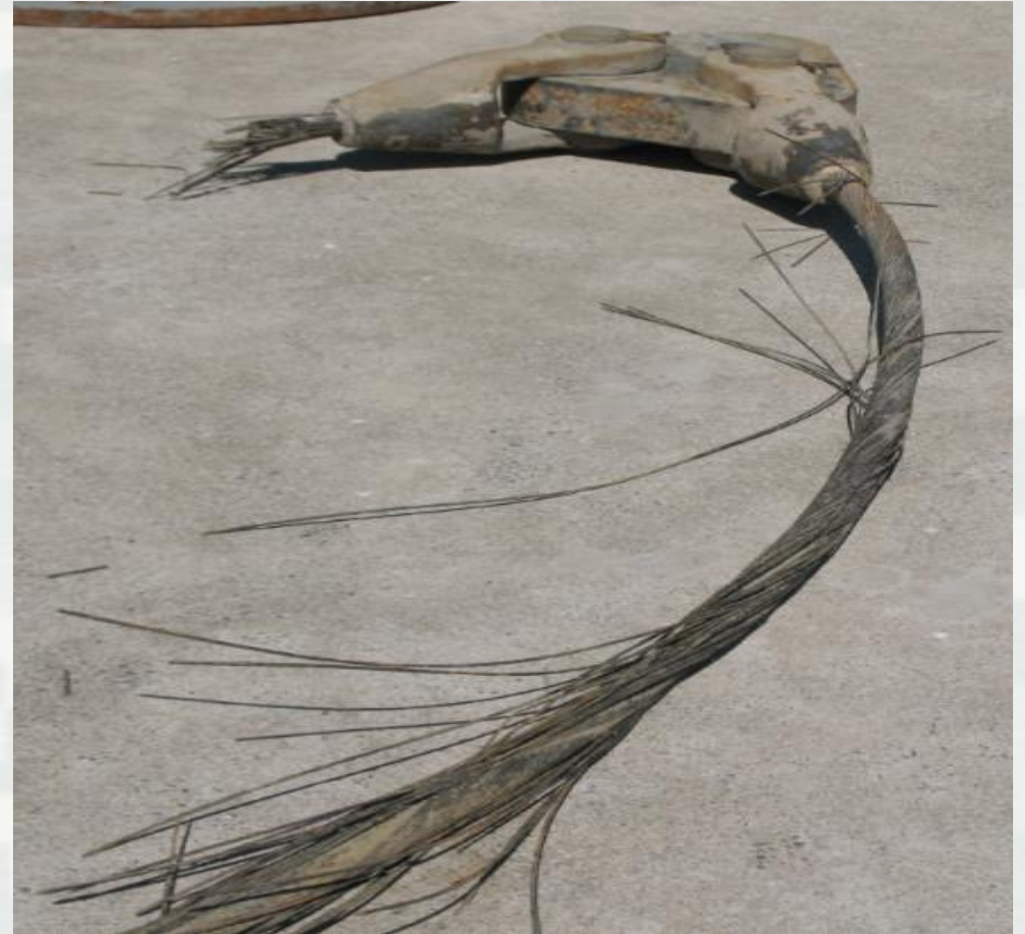
2020 Lower Monumental broken floating guide wall cable
